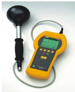
Fig. 4.2. The meter of electromagnetic field voltage (Narda NBM-550).
