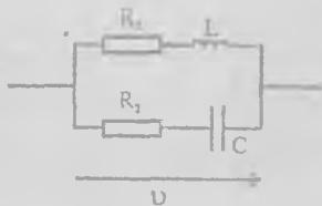
$$y = G = \frac{R_1}{R_1^2 + R_2^2} + \frac{R_2}{R_2^2 + R_2^2}$$
