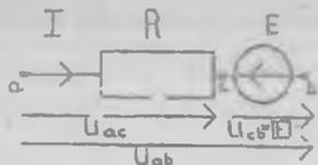
$$I = U_{ac}/R = (\varphi_a - \varphi_c)/R = (\varphi_a - (\varphi_b + E))/R =$$
