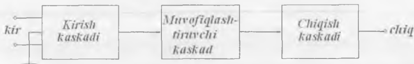
9.15-rasm. Uch kaskadli OK funksional sxemasi.
