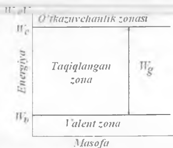
1.2-rasm. Qattiq jism zonalar energetik diagrammasi.
