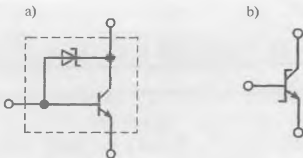
11.11-rasm. Shottki barerili tranzistor (a) va uning shartli belgisi (b).
