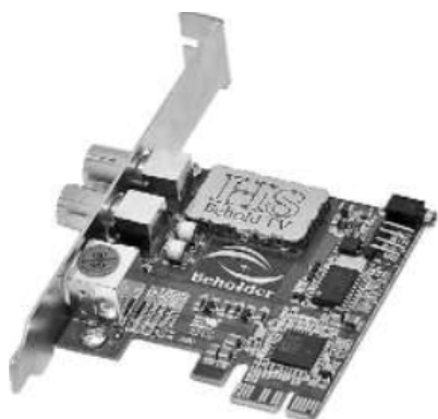
2.21-rasm. Ichki PCI – Express TV/FM – tyuner.
