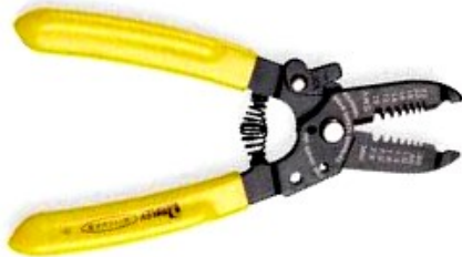
17.17-rasm. Optik tola bufer qatlamini ajratuvchi stripper asbobi.
