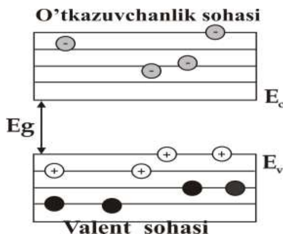
2-rasm. Xususiy yarim o'tkazgichning energetik diagrammasi
