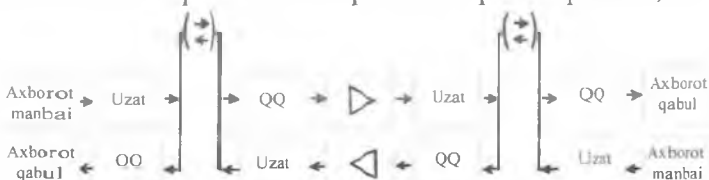
1.4-rasm. Radioreleli aloqa liniyasining qurilishi
