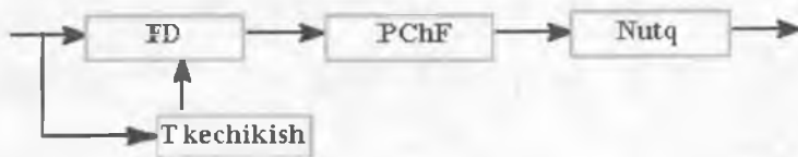
5.8-rasm. NFM signalni differensial-kogerent detektirlash
