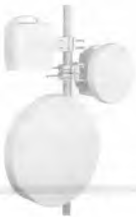
4.9-rasm. Antenna tayanchidagi MINI-LINK apparaturasi- ning modullari
