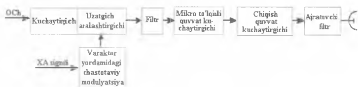
6.2-rasm. RRL uzatkichning funksional sxemasi
