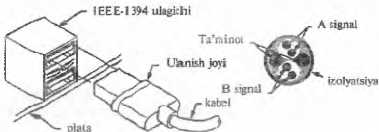
3.27-rasm. IEEE-1394 shinasining kabeli, ulanish joyi va ulovchisi.
