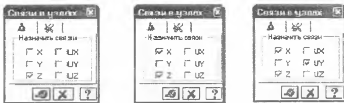
3.2-rasm. Tayanch bog'lanishi turlari: a) sharnirli qo'zg'aluvchan tayanch; b) sharnirli qo'zg'almas tayanch; v)sharnirsiz qo'zg'almas tayanch.
