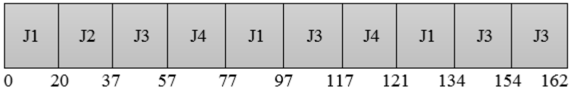
2.22- rasm. RR algoritmini qo‘llanishiga misol ( q = 20 )
