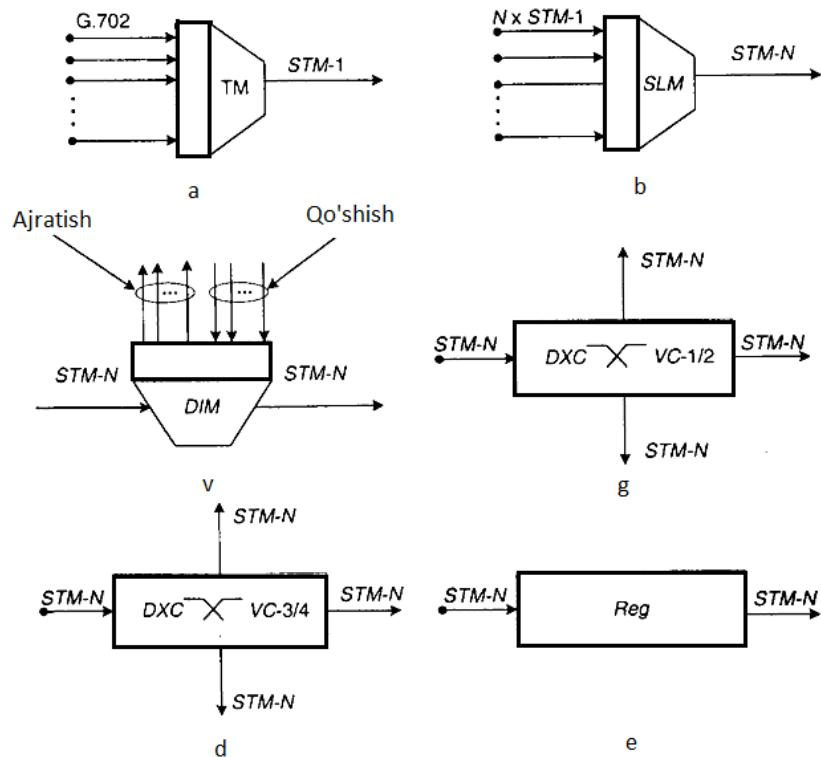
5.1 – rasm. TM (a,b), ADM (c), DXC(g,d) va regeneratorlarning shartli (e) belgilanishlari
