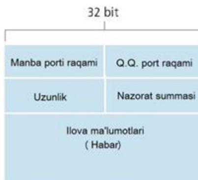
16.3-rasm. UDP segmentining tuzilishi
