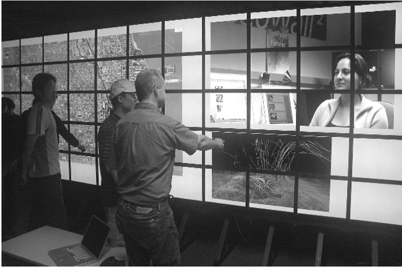
Figure 2.2. “LambdaVision” 100-megapixel (55-LCD panel) tiled.
