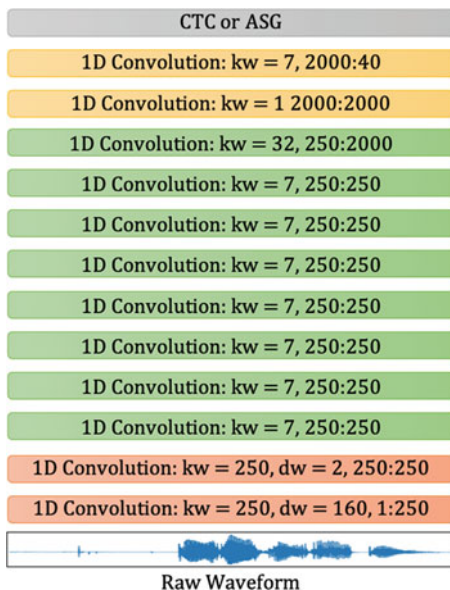
Fig. 12.6: Wav2Letter architecture for recognition on a raw waveform. The first layer is not included when training on MFCCs instead of the raw waveform. The convolutional parameters are organized as (kw, dw, \text{dim ratio}) , where kw is the kernel width, dw is the kernel stride, and dim ration is the number of input dimensions to the number of output dimensions
