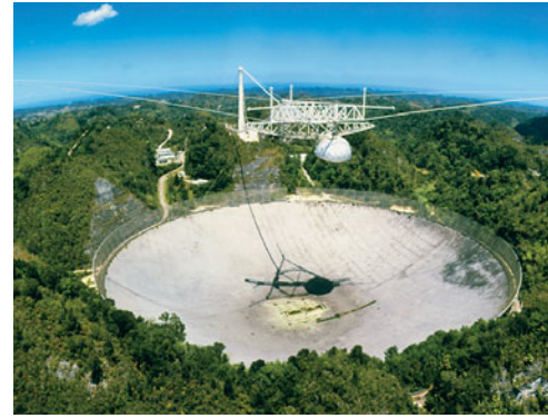
FIGURE 25–33 The 300-meter radiotelescope in Arecibo, Puerto Rico, uses radio waves (Fig. 22–8) instead of visible light.
