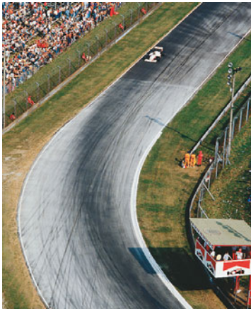
FIGURE 5-12 Race car heading into a curve. From the tire marks we see that most cars experienced a sufficient friction force to give them the needed centripetal acceleration for rounding the curve safely. But, we also see tire tracks of cars on which there was not sufficient force—and which unfortunately followed more nearly straight-line paths.
