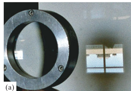
FIGURE 23-38 (a) A converging lens can form a real image (here of a distant building, upside down) on a white wall. (b) That same real image is also directly visible to the eye. [Figure 23-31d shows images (graph paper) seen by the eye made by both diverging and converging lenses.]
