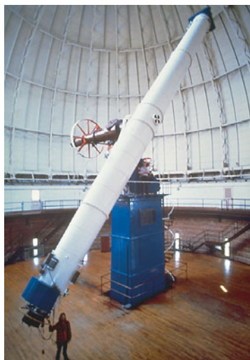
FIGURE 25–21 This large refracting telescope was built in 1897 and is housed at Yerkes Observatory in Wisconsin. The objective lens is 102 cm (40 inches) in diameter, and the telescope tube is about 19 m long. Example 25–8.
