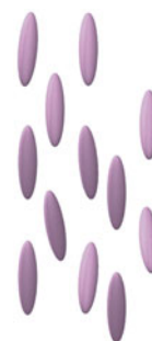
FIGURE 24–50 Liquid crystal molecules tend to align in one dimension (parallel to each other) but have random positions (left-right, up-down).
