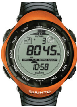
FIGURE 24-52 Watch-face LCD display with altimeter. The black segments or pixels have a voltage applied to them. Note that the 8 uses all seven segments (pixels); other numbers use fewer.
