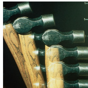
FIGURE 4-7 A hammer striking a nail. The hammer exerts a force on the nail and the nail exerts a force back on the hammer. The latter force decelerates the hammer and brings it to rest.
