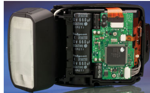
FIGURE 17-20 A camera flash unit. The 660- \mu\text{F} capacitor is the black cylinder.
