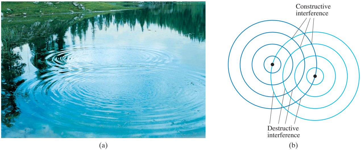
FIGURE 11-38 (a) Interference of water waves. (b) Constructive interference occurs where one wave's maximum (a crest) meets the other's maximum. Destructive interference ("flat water") occurs where one wave's maximum (a crest) meets the other's minimum (a trough).
