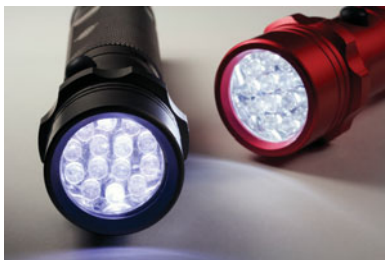
FIGURE 29–35 LED flashlights. Note the tiny LEDs, each maybe \frac{1}{2} cm in diameter.
