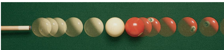
FIGURE 7-14 In this multi-flash photo of a head-on collision between two balls of equal mass, the white cue ball is accelerated from rest by the cue stick and then strikes the red ball, initially at rest. The white ball stops in its tracks, and the (equal-mass) red ball moves off with the same speed as the white ball had before the collision. See Example 7-7, part (b).
