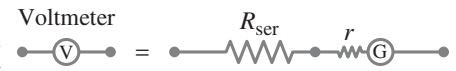
FIGURE 19–32 A voltmeter is a galvanometer in series with a resistor with high resistance, R_{\text{ser}} .
