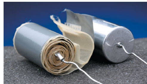
FIGURE 17–18 A cylindrical capacitor, unrolled from its case to show the dielectric between the plates. See also Fig. 17–13b.
