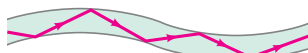
FIGURE 23–29 Light reflected totally at the interior surface of a glass or transparent plastic fiber.
