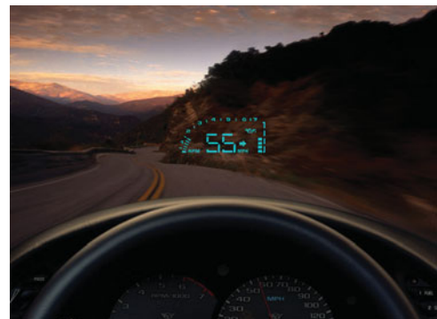
FIGURE 29–39 Head up displays on curved windshields can use curved OLEDs to show, for example, your speed without having to look down at the speedometer.
