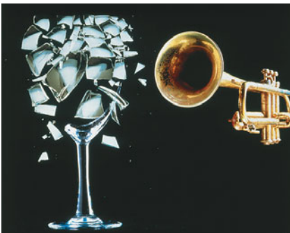
FIGURE 11–19 This goblet breaks as it vibrates in resonance to a trumpet call.
