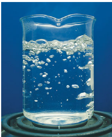
FIGURE 13–25 Boiling: bubbles of water vapor float upward from the bottom (where the temperature is highest).
