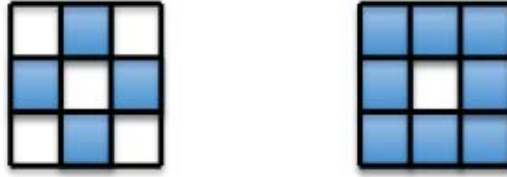
Figure 2-2: Pixel groupings defining commonly used neighborhoods with respect to the center. (Left) 4-point neighborhood. (Right) 8-point neighborhood.
