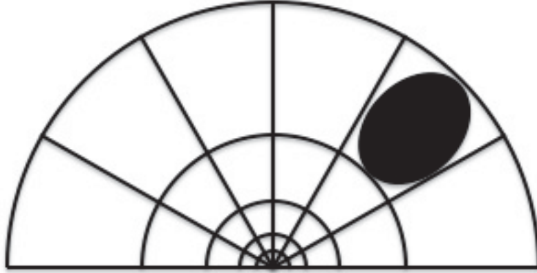
Figure 3-4: Partition of the spatial frequency plane into 30 channels for the Homogeneous Texture Descriptor.
