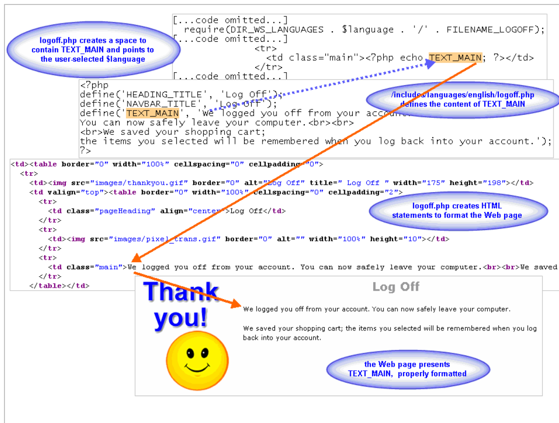
Figure 49: Multiple layers of substitution into placeholders allow human language to be presented with other user-specific data.
