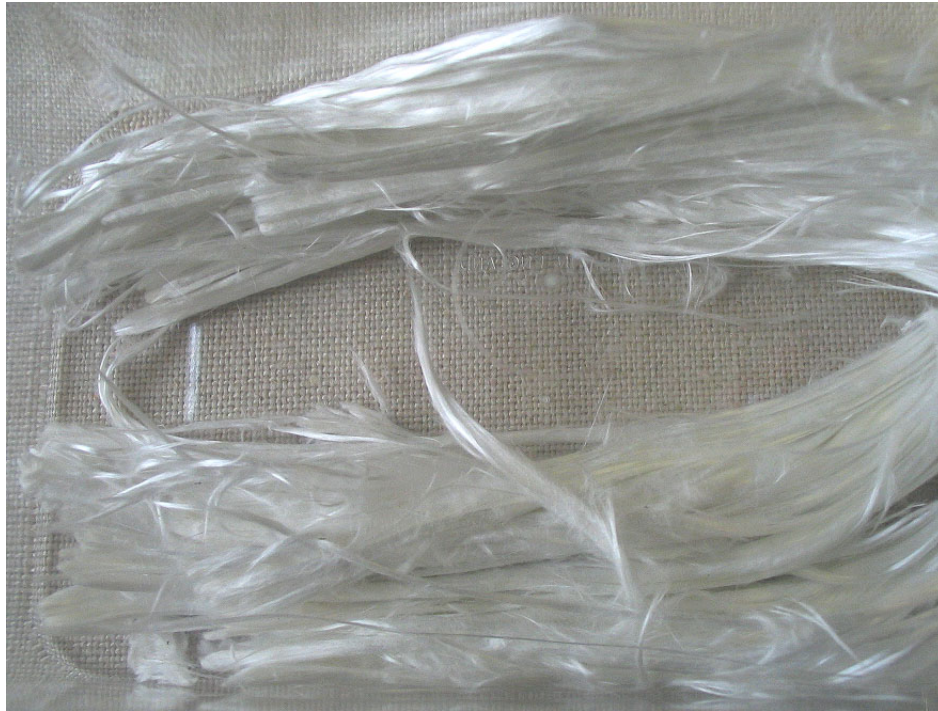
Figure 1.1: A photograph of asbestos fibers used to weave insulation material. Note the long, thin crystal shape. Source: Wikimedia, “Asbestos fibres,” accessed January 31, 2012 ( http://commons.wikimedia.org/wiki/File:Asbestos_fibres.jpg ; Wikimedia Commons is a media file repository making available public domain and freely-licensed educational media content to everyone).
