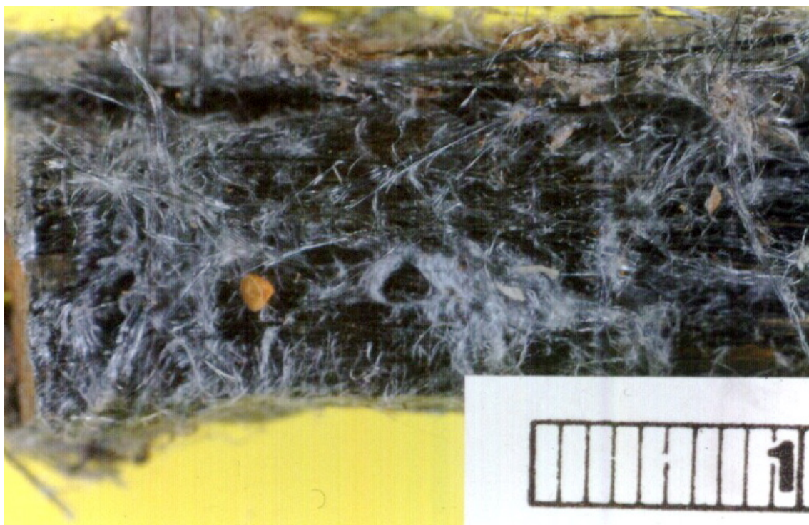
Figure 1.2: A sample of blue (crocidolite) asbestos from Wittenoom in Western Australia. Note the fibrous and spindle-like nature of the mineral. The ruler is 1 centimeter. Source: Wikimedia, “Blue asbestos (teased),” accessed January 31, 2012 ( http://commons.wikimedia.org/wiki/File:Blue_asbestos_(teased).jpg ).
