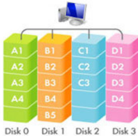
Figure 1. Just a Bunch of Disks. [11]
