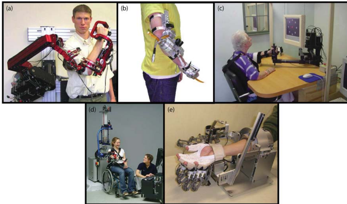
Figure 1.5: The rehabilitation actuation systems at the upper extremity: (a) The cable-actuated dextrous exoskeleton for neurorehabilitation (CADEN) [60], (b) WOTAS exoskeleton for tremor suppression [67], (c) MIT-MANUS planar upper extremity rehabilitation robot [46], [47], (d) ARMin exoskeleton for stroke patient therapy [53], and (e) The hand motion assist robot [37].
