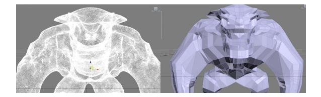
Figure 16. Compared to the high-density original mesh (left) the new low-density version is more suited for fully articulating body movements.
