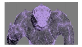
Figure 3. An example of the varying vertex concentration within a Leo-generated digital mesh. The highly detailed portions of the face and head contain much more topographical geometry than the flat portions of the torso.
