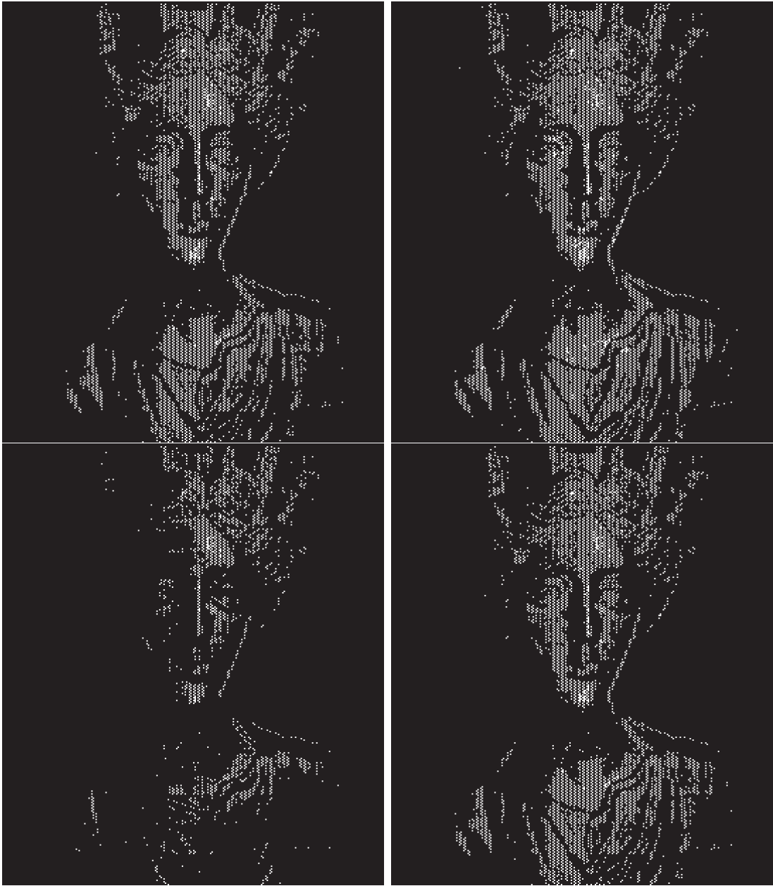
Figure 3.11: Printed masks and simulated outputs for a fixed viewpoint and fixed lighting direction. a) Standard halftone. b) Echo compensated halftone; c) Simulation output of halftone pattern in (a). d) Simulation output for halftone pattern in (b). As in Figure 10, the simulation in (d) approximates (a) more closely than the simulation in (c) does.
