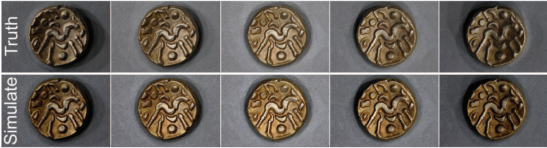
Figure 3.13: To validate our design using an overlay across multiple lighting directions we simulate the effect of moving a light across a 90 degree arc of illumination angles. Five frames from the resulting sequence are shown here. The average RMS error across all frames is 5.0%, and nowhere does the error exceed 6.3%, remaining relatively consistent across the full range of lighting angles.
