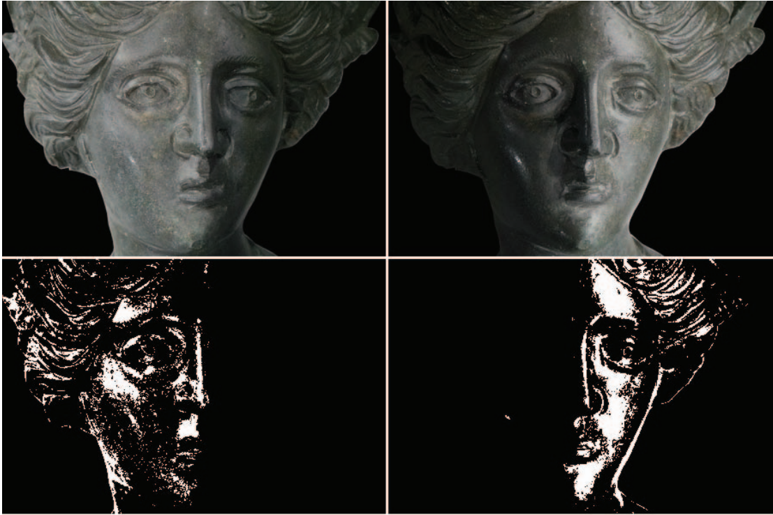
Figure 3.7: Simply thresholding the grayscale reflectance function (top) to black and white (bottom) , produces images which relight correctly, but with the expected quantized binary response.
