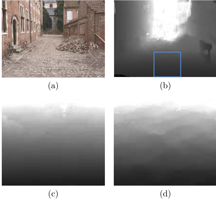
Figure 4.6: (a) Original image. (b) Depthmap computed using our multi-sweep method. Close-ups are shown for the marked area. (c) Close-up of the multi-sweep depthmap. (d) Close-up of the fronto-parallel sweep depthmap. Notice the staircase artifacts.
