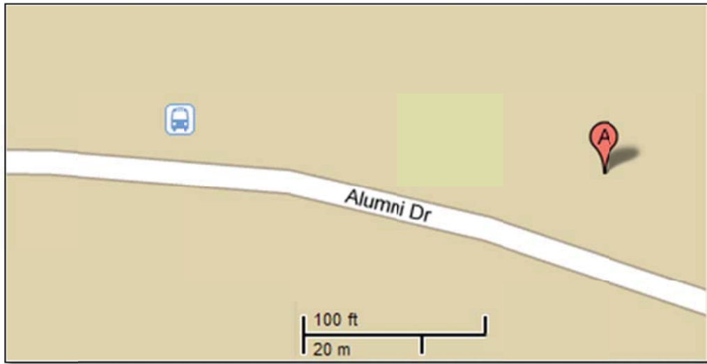
Figure 60 - Some TAD alerts were given early or late due to incorrectly geocoded bus stops, where the actual bus stop position (marker "A") differed from the database location of the bus stop (blue bus icon)
