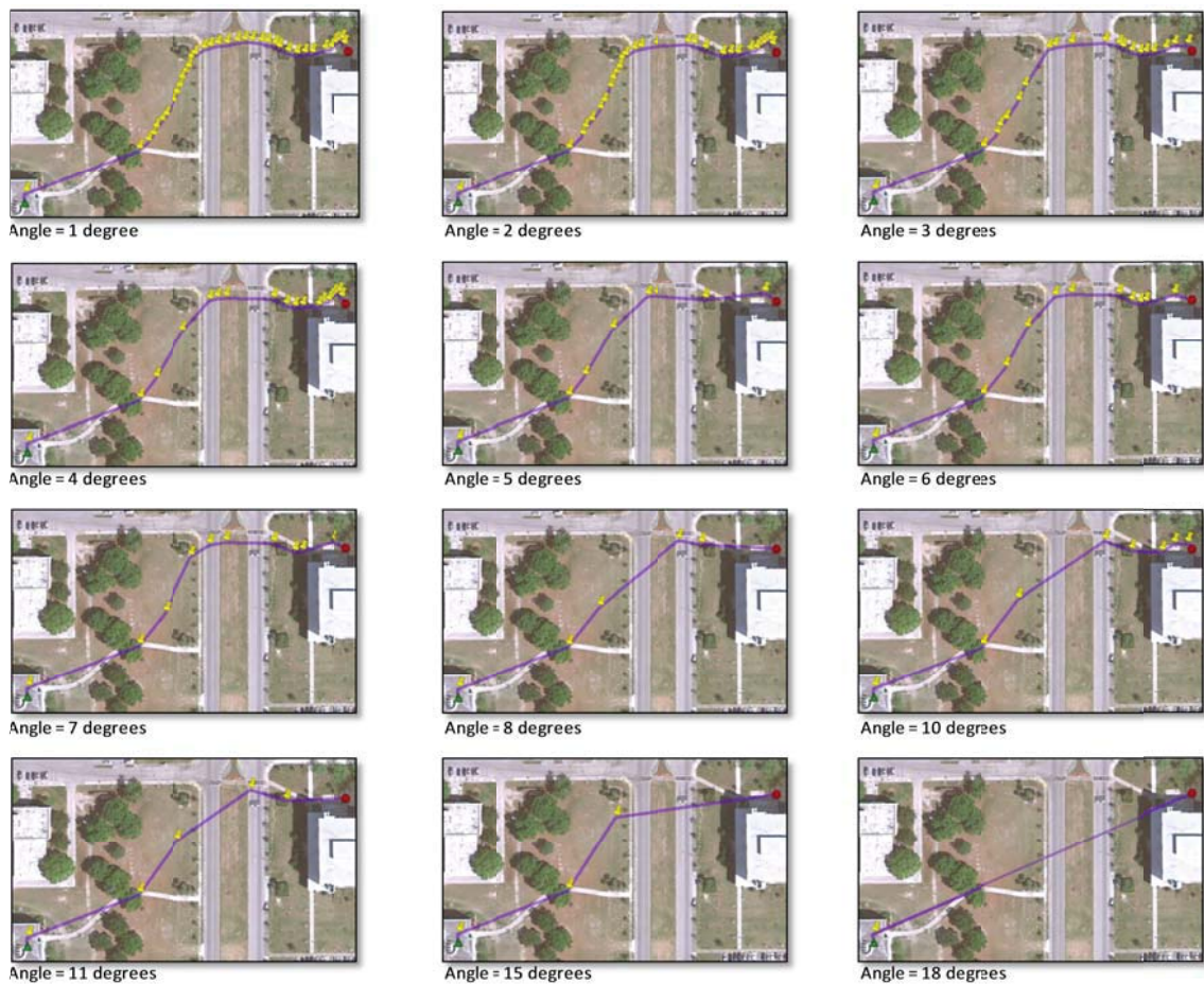
Figure 44 - Running the Critical Point Algorithm with increasing angle thresholds gradually reduces the number of points that represent the line, which increases the distance error percentage
