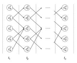
Figure 4. Change propagation network of five components
