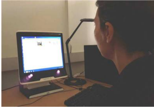
Figure 1 : Remote eye tracker. Eye cameras are embedded between LED lights seen below screen image
