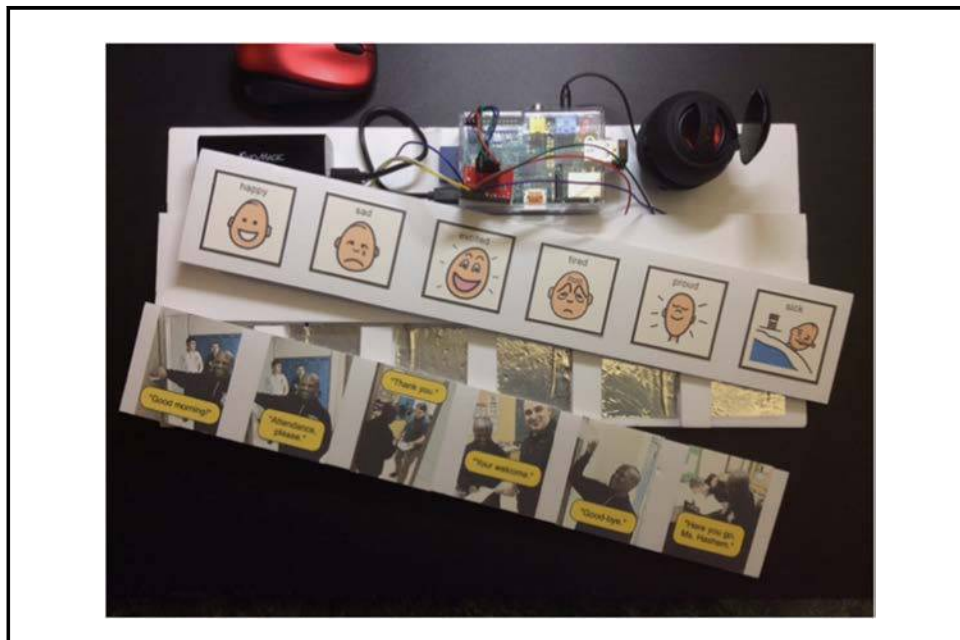
Plate 2 Prototype 2, TalkBox, consists of a Raspberry Pi connected to a capacitive touch sensor, speakers and a hand-made foam board with aluminium foil touch-switches
