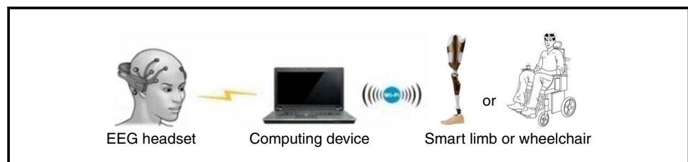
Figure 4 The use of thought control to operate smart assistive mobility devices
