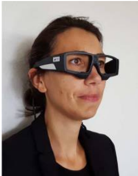
Figure 2: Eye tracking glasses with eye cameras and LED lights embedded in lower part of frame
