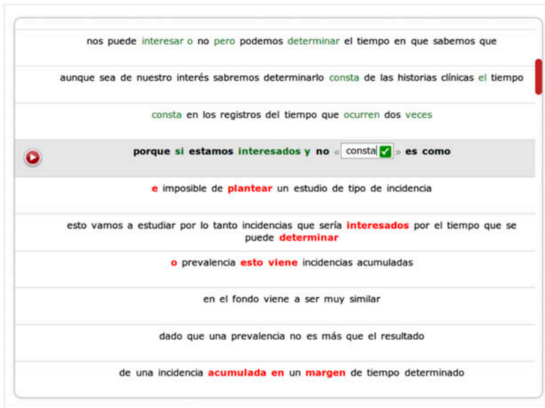
Figure 4. Screenshot of the transcription interface in computer-aided interaction mode. Low-confidence words appear in red and supervised low-confidence words in green. The word being edited in this example is opened for supervision, and the text box can be expanded to the left or right by clicking on << or >>, respectively. Clicking the green check button to the right of the text box confirms the word as correct.
