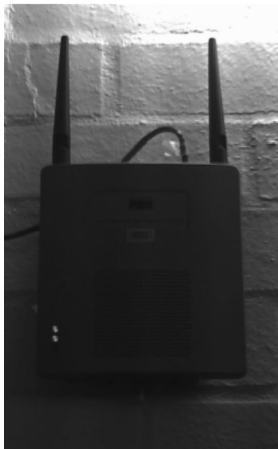
Figure 2 Dual-monopole array mounted close to a reflecting wall in a WLAN base station
