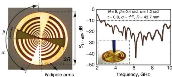
**Fig. 1** Planar LP antenna and its measured  $S$ -parameter response using  $100 \Omega$  differential probe (shown in inset)
