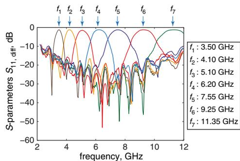
**Fig. 3** Identification of centre frequencies of rejection bands, corresponding to each dipole arm of LP aperture
