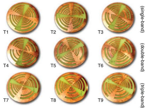
**Fig. 2** Various fabricated prototypes of printed LP antenna with single, double or triple band-rejection response
