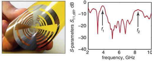
**Fig. 5** Photograph of LP tag antenna printed on flexible substrate and its corresponding  $S$ -parameter response to illustrate RFID code
