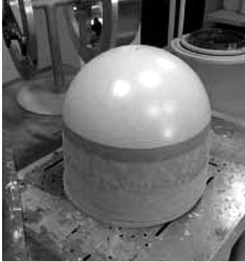
Fig. 5. Model of three-layer heat-shield screen made from inorganic glass-reinforced plastic.
