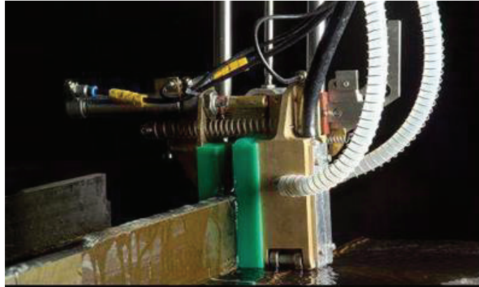
FIGURE 8. Phased array stringer inspection tool.
