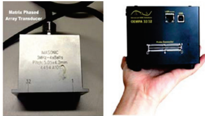
FIGURE 3. Matrix array probe and OEMPA UT electronics.
