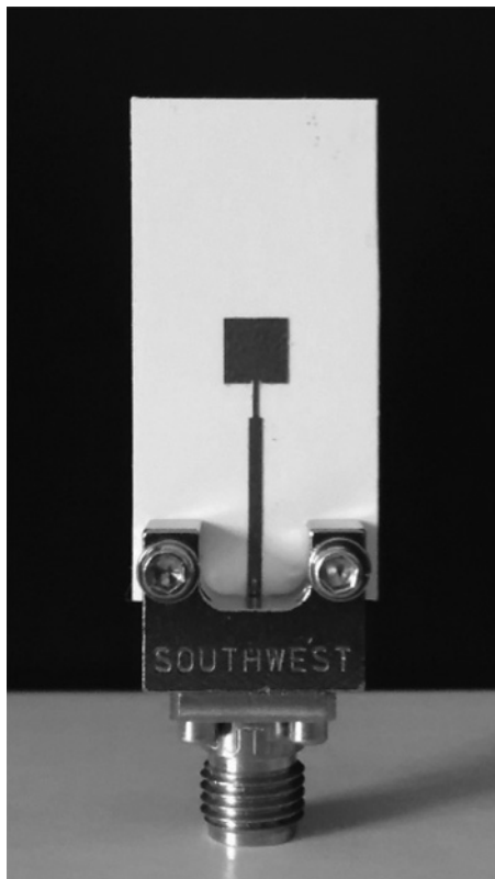
Fig. 6 Photographs of the fabricated radiating element (i.e. single patch) with the coaxial to microstrip launcher used during the measurements
