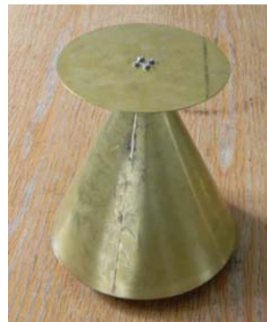
FIGURE 2. Prototype B of the disccone antenna element with feeding from the top (cone) side.
