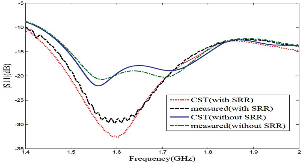
**Figure 2.** Measured and simulated input reflection coefficients of antenna array with and without SRR structures. (color figure available online)
