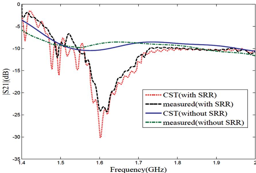
**Figure 7.** Measured and simulated mutual coupling of antenna array with and without SRR structures. (color figure available online)
