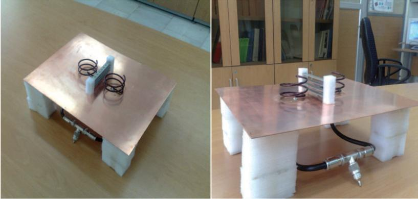
**Figure 6.** Fabricated short helical antenna array with SRRs installed between the elements. (color figure available online)
