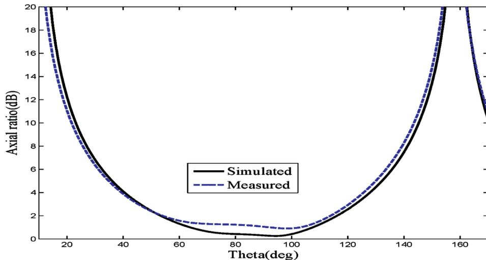
**Figure 3.** Measured and simulated ARs versus the elevation angle at frequency of 1.575 GHz. (color figure available online)
