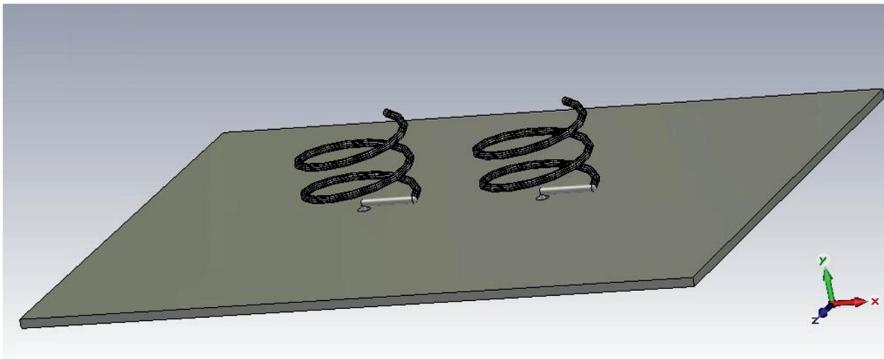
**Figure 1.** Layout of the  $1 \times 2$  short helical antenna array with rectangular ground plane. (color figure available online)
