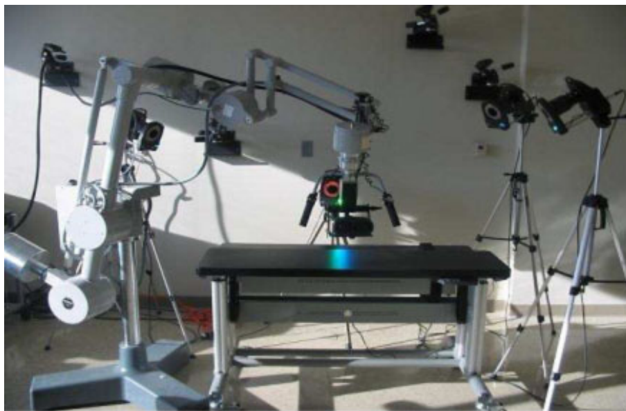
Figure 7 VICON Cameras on tripods and Microscope and binocular display and the end of the Microscope arm (Previous AR setting).
