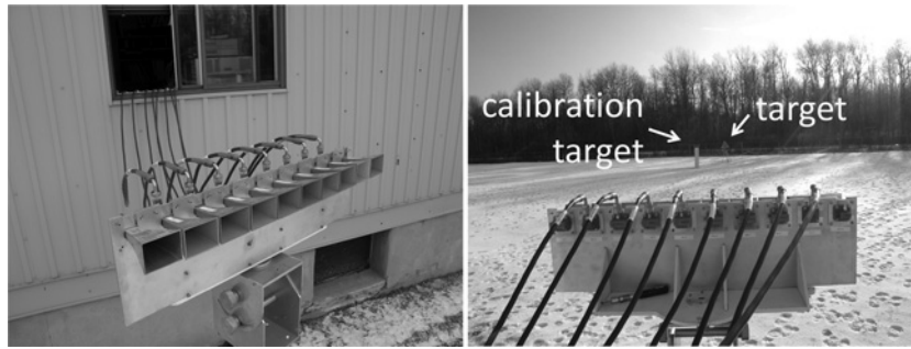
Fig. 2 Photographs of the linear array (left) and the setup (right) for the time-division coherent MIMO experiment
