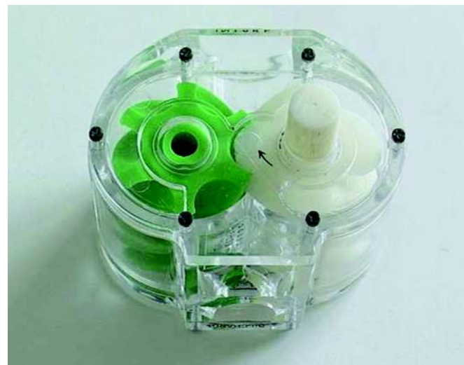
Figure 7 A photograph of a simplified model of a twin-screw compressor in a transparent casing.
