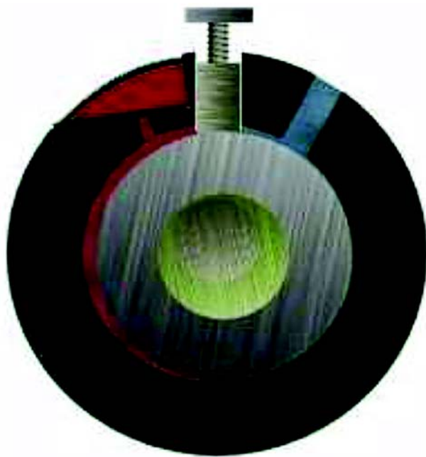
Figure 4 A computer-generated model of a rolling piston with correct dimensions.
