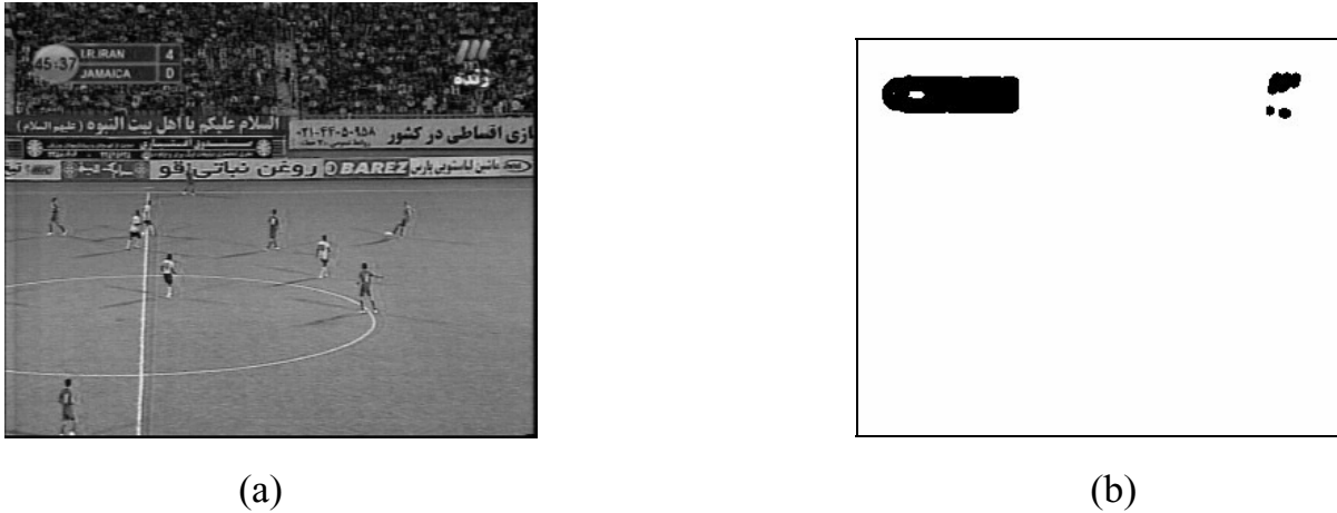
Fig. 3. Bi-level image of caption, (a) A frame of soccer game. (b) Bi-level image of caption.
