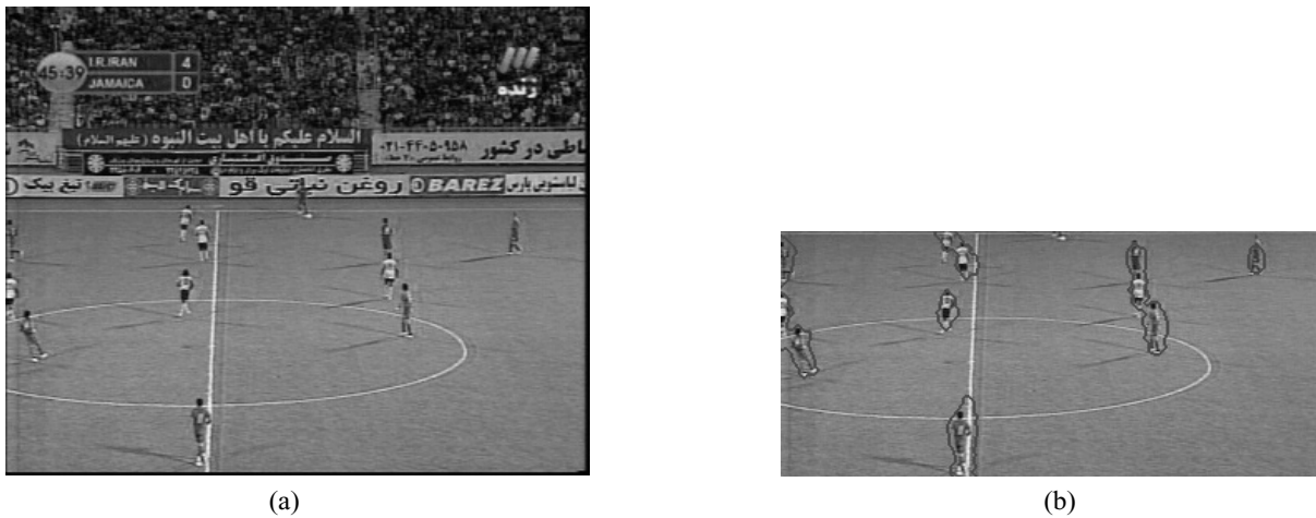
Fig. 10. An image with artificial lighting condition. (a) Original image notice the shadows created by the players. (b) Obtained image by applying Bi-level image of players on original image.
