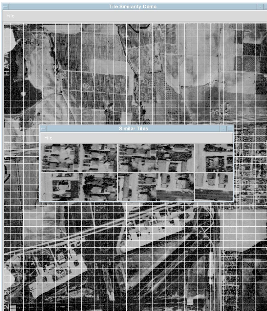
Fig. 13. Each aerial photo is partitioned into 40 \times 40 small image blocks and indexed by Gabor filters. After the user clicks on an image block, the Java-based system pops out a separate window to display the image block (the top-leftmost image in the popped-out window) and its similar blocks (seven similar image blocks displayed in ranked order from left to right and top to bottom)
