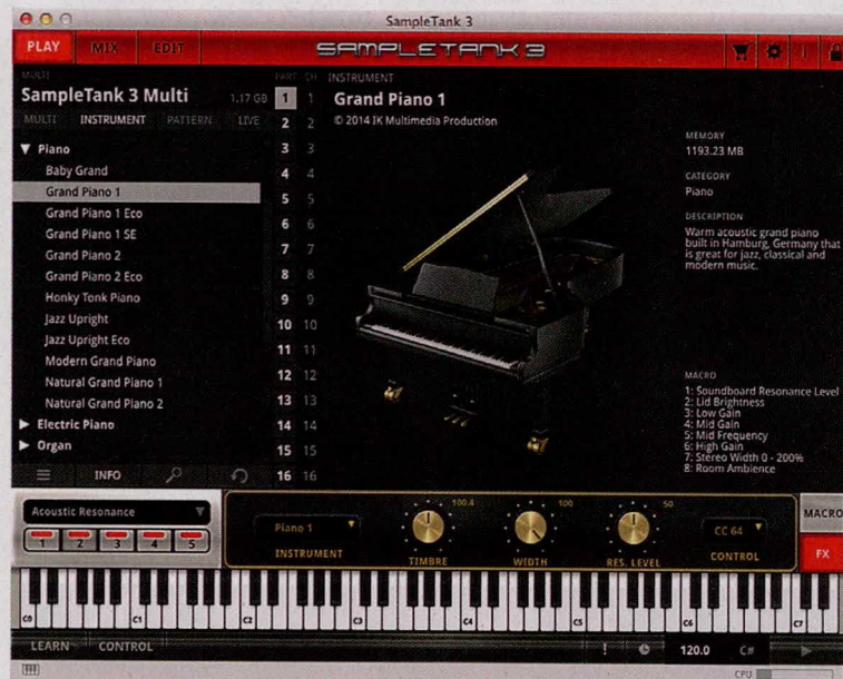
Fig. 1. SampleTank 3's Play page gives you easy access to the browser and all 16 Parts in its multitimbral architecture.
