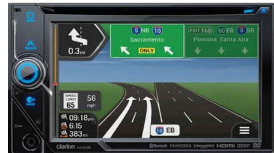
The double-DIN NX-405 navigation/multimedia head unit has an HDMI input to mirror the displays of a connected Android or Apple phone.
