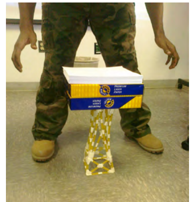
Figure 1. A. A tower supporting a load of 5.7 kg.
