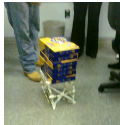
Figure 1. B. A tower collapsing under a load of 13.6 kg
