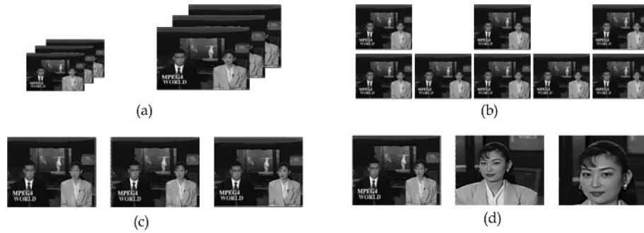
Fig. 6. An illustration of various scalable coding schemes: (a) spatial scalability; (b) temporal scalability; (c) quality scalability; and (d) attention scalability.
