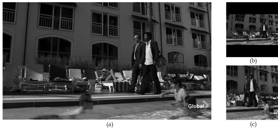
Fig. 10. Example of video retargeting: (a) original 624 \times 352 video; (b) a 120 \times 120 video by simply resizing; and (c) a 120 \times 120 video by retargeting with visual saliency.
