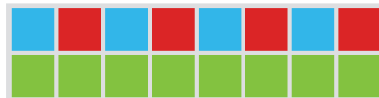
Bilinear sensor with Bayer pattern
