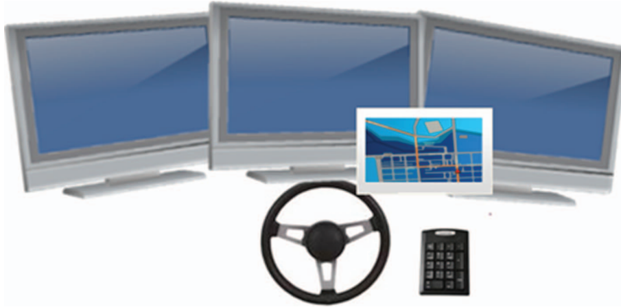
Figure 1. An illustration of the experimental system including: the three screens of the driving simulator and steering wheel, the small screen presenting the maps in the navigation system, and the numeric keypad used for answering navigational questions and ratings.
