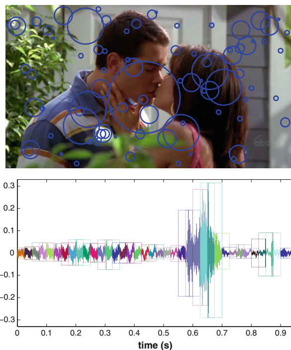
Fig. 5 Local audio-visual features. Top Spatio-temporal interest points (STIP) are used as basis for visual features. A HOG/HOF descriptor is computed for each STIP. Bottom Audio signal is divided into overlapping frames . In this example, the signal is divided in frames of 0.05 s overlapping 0.025 s. Features are extracted over each audio frame. Then, each resulting feature vector is assigned to a word of the corresponding dictionary
